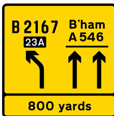
**Figure 8.5** Typical Diagram 7244 sign
