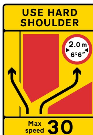
Figure 8.4 Typical Diagram 7243 sign
