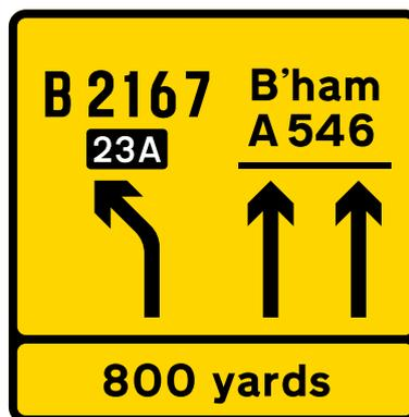
**Figure 8.5** Typical Diagram 7244 sign
