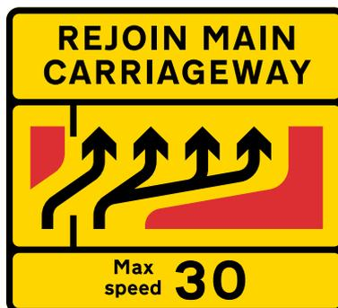
Figure 8.6 Typical Diagram 7245 sign
