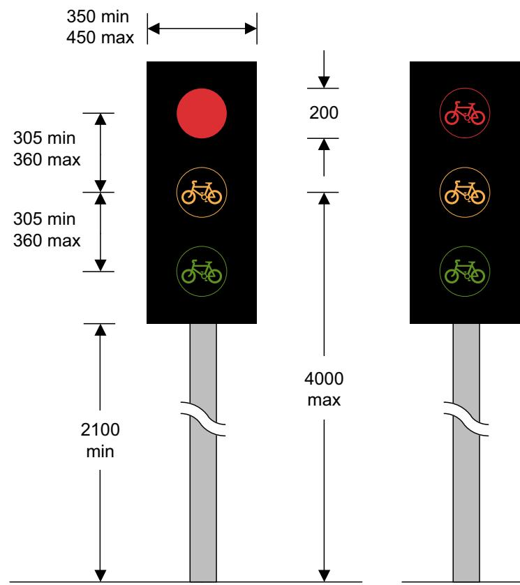
**Figure 12-2** Diagram 3000.2 (S14-2-3), alternative types
