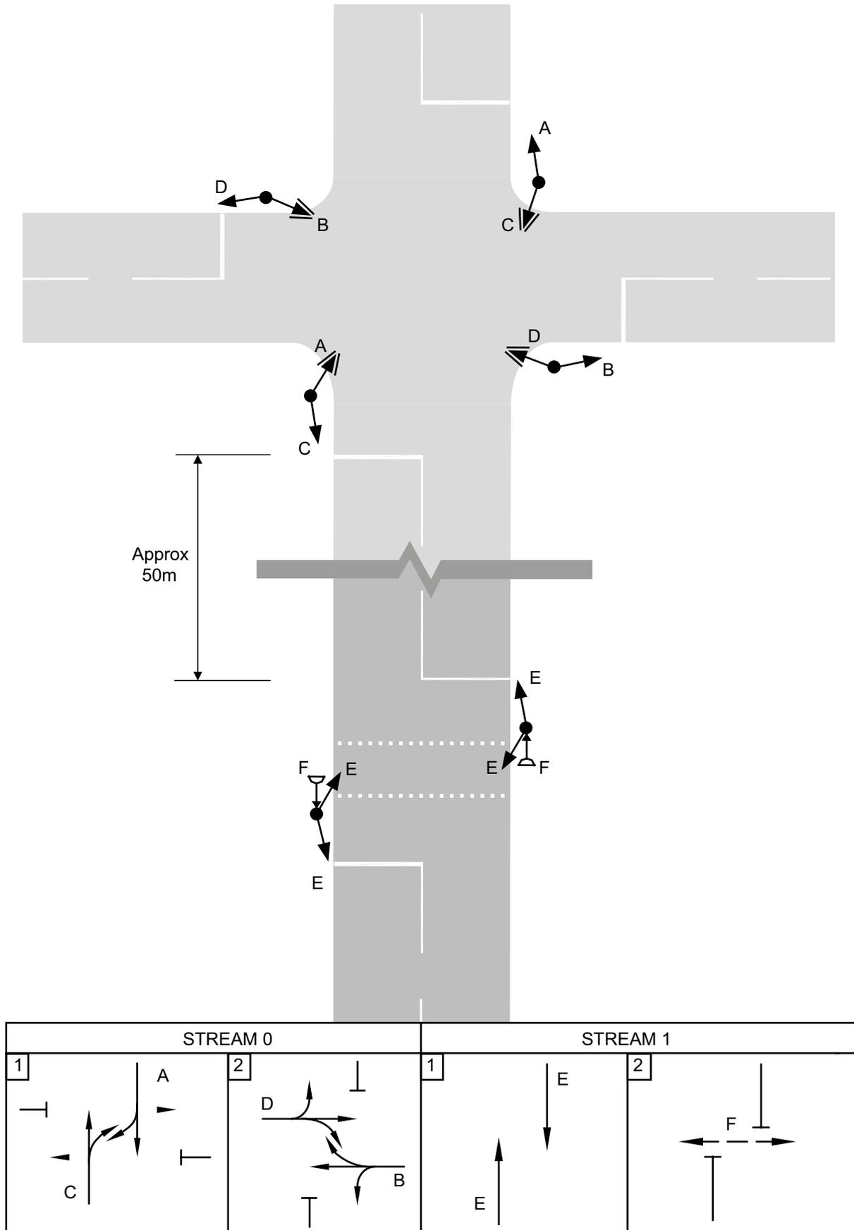
**Figure 11-7** Diagram showing indicative layout and staging for a displaced pedestrian facility
