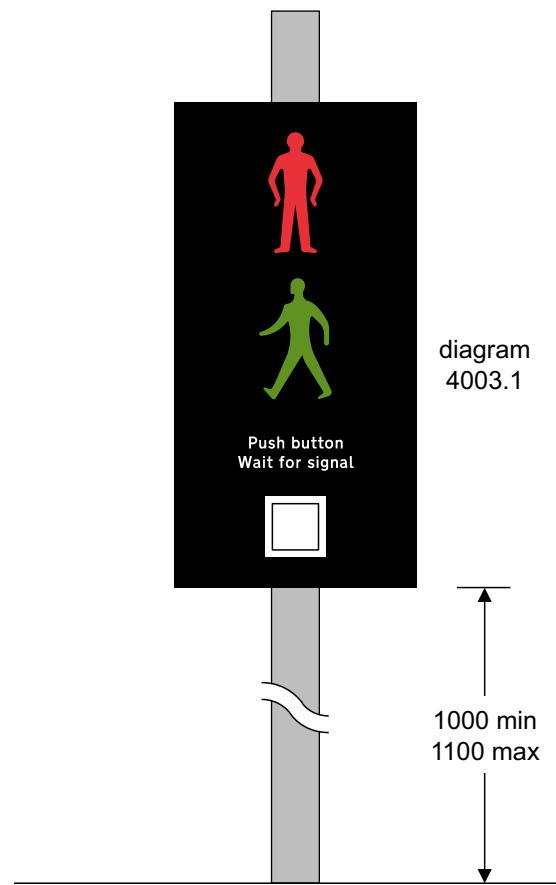
**Figure 11-2** Pedestrian demand unit to diagram 4003.1 (S14-2-13)
