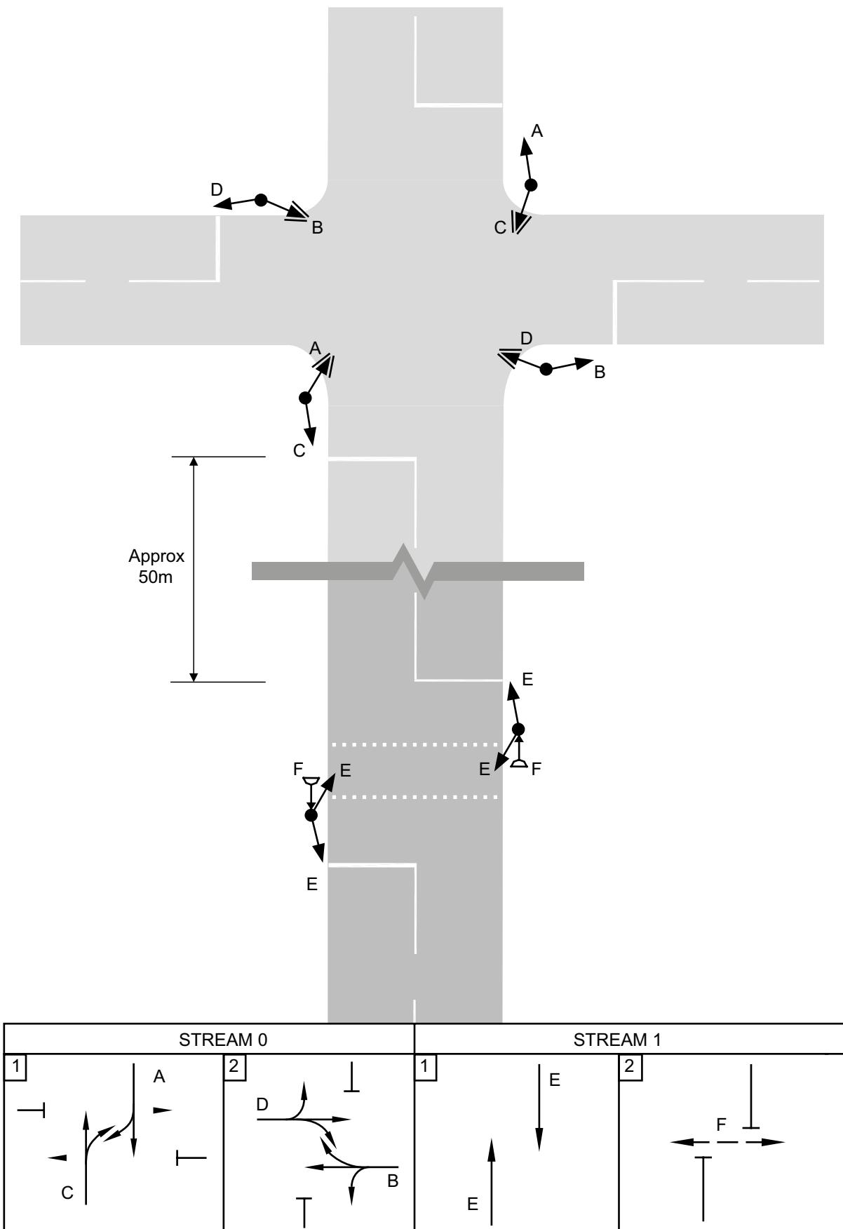
**Figure 11-7** Diagram showing indicative layout and staging for a displaced pedestrian facility
