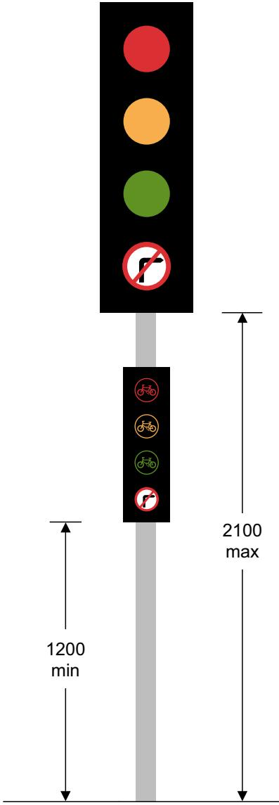
**Figure 12-4** Diagram 3000 (S14-2-1) shown in combination with low-level cycle signals and an optional regulatory box sign
