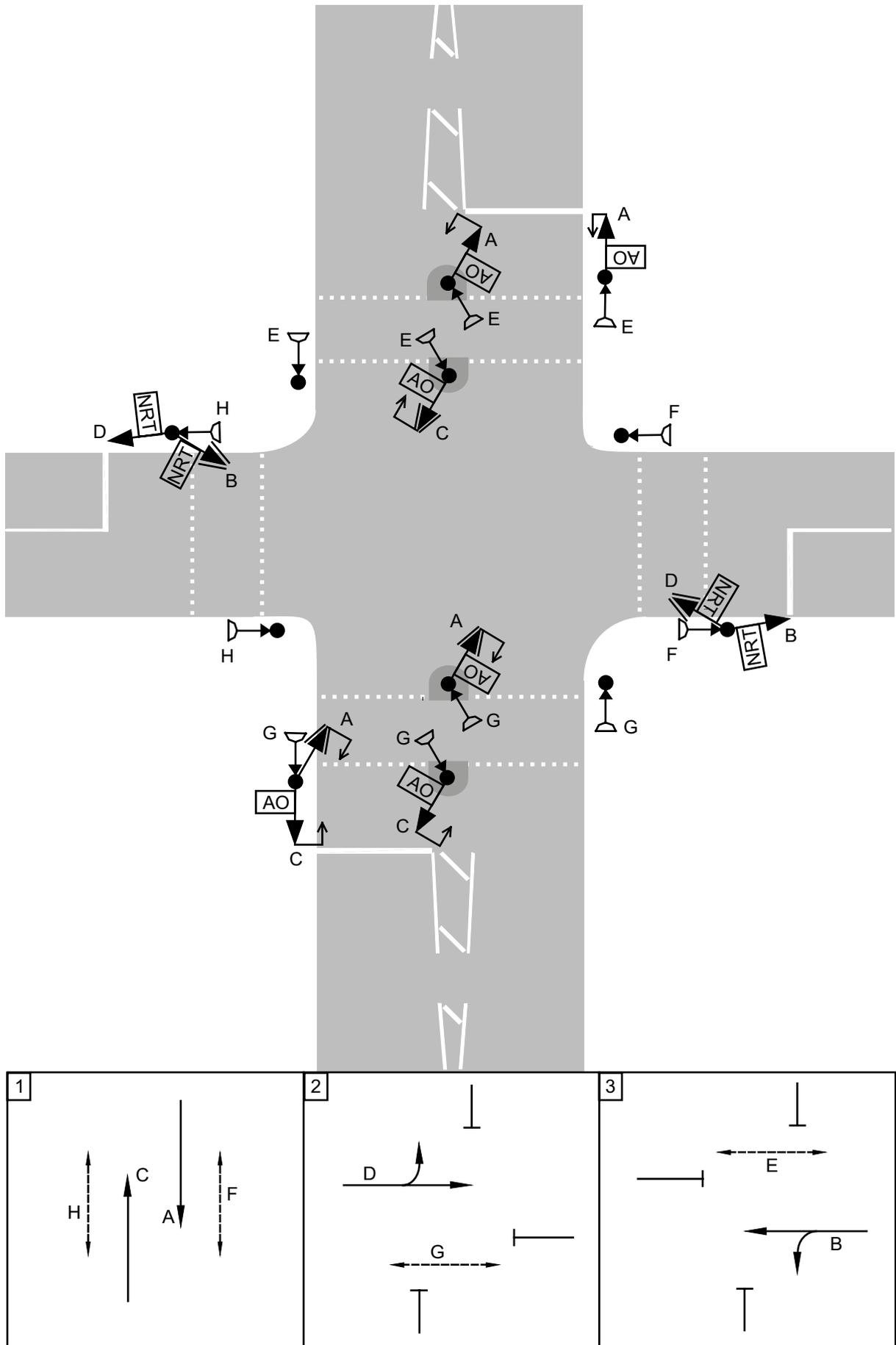
Figure 11-5 Walk with traffic pedestrian facility
