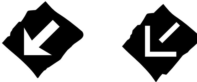
**Figure 26-4** Diagrams 5005 and 5005.1 (S14-2-34) Lane closed ahead and vehicular traffic should move to the next lane on the left (Alternative types)
