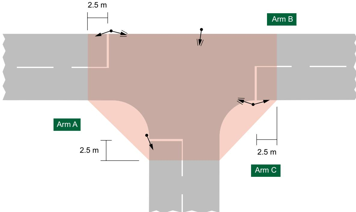
**Figure 2-1** Diagram showing a Junction Intervisibility Zone (without crossings) in relation to the road layout
