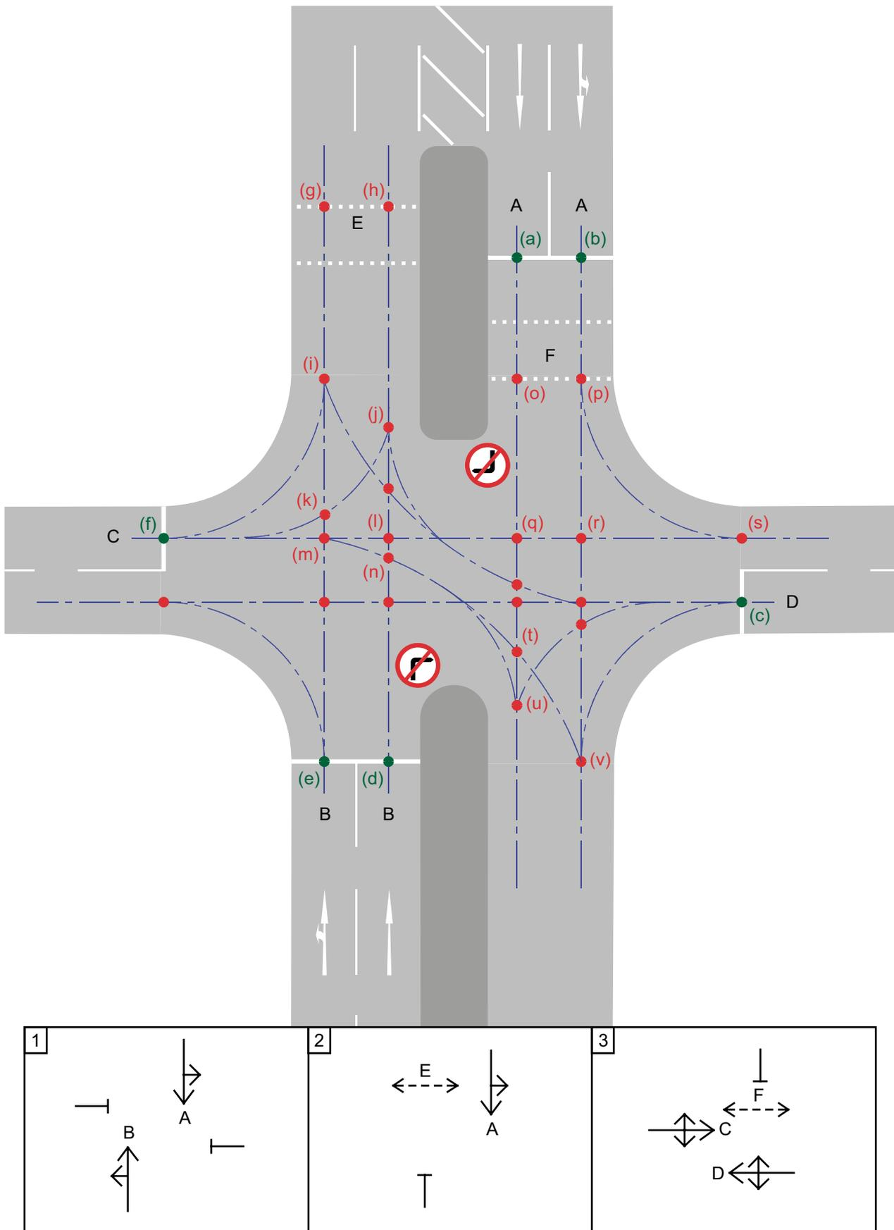
**Figure 6-3** Layout diagram showing probable collision points for movements at a typical crossroad junction
