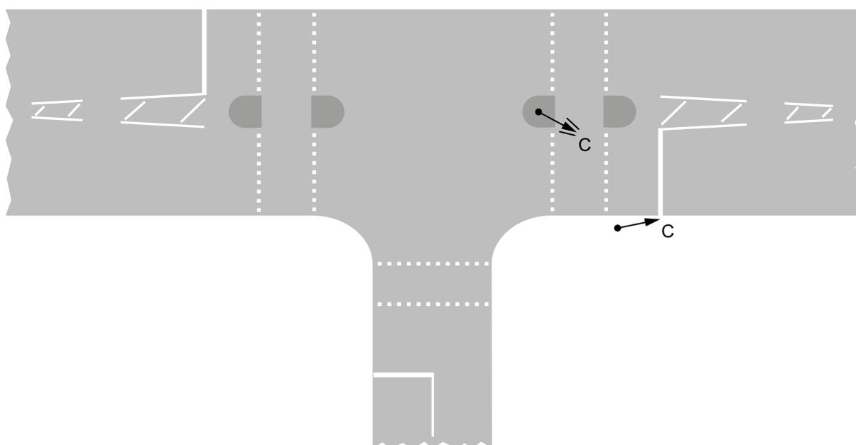
**Figure 3-3** Layout diagram showing the positions of a primary signal head plus a closely associated secondary signal head
