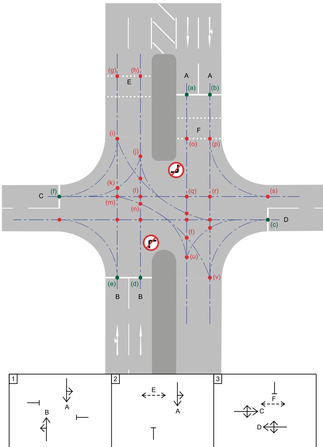
**Figure 6-3** Layout diagram showing probable collision points for movements at a typical crossroad junction
