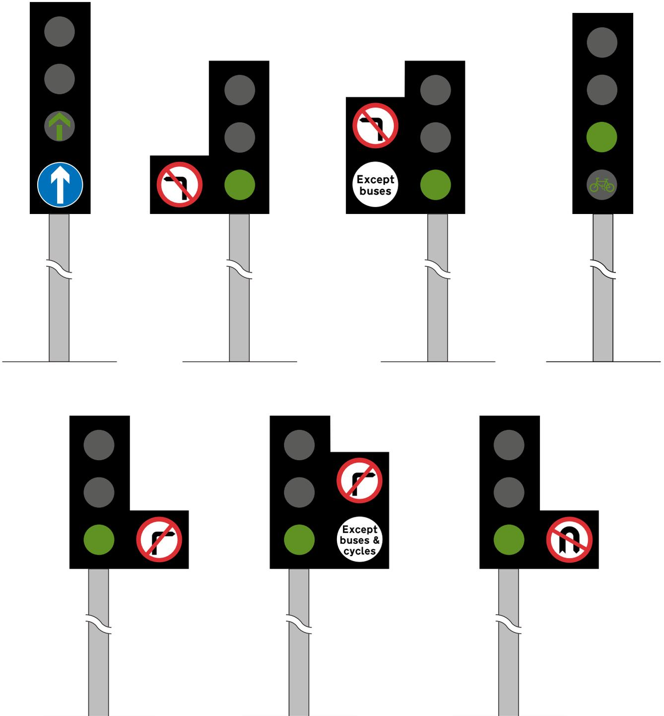
**Figure 5-1** Alternative signal head layouts showing common regulatory box sign arrangements and exception plates
