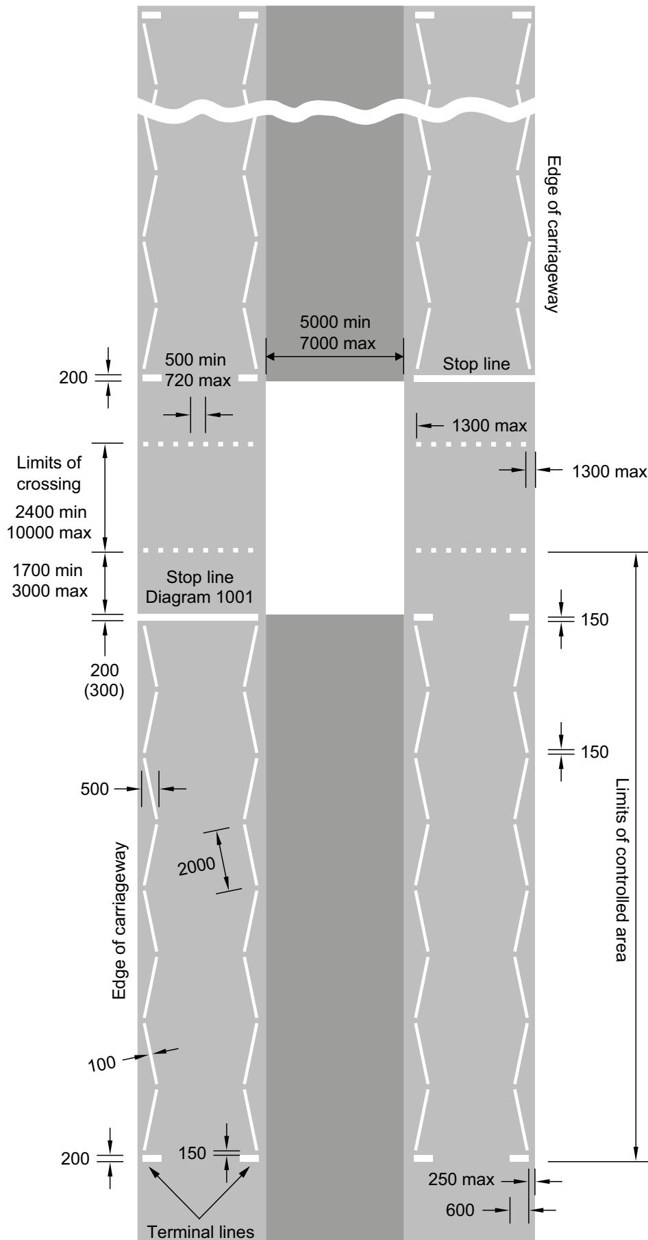
**Figure 18-1** Diagram showing suggested layout for an in-line crossing operating in two stages
