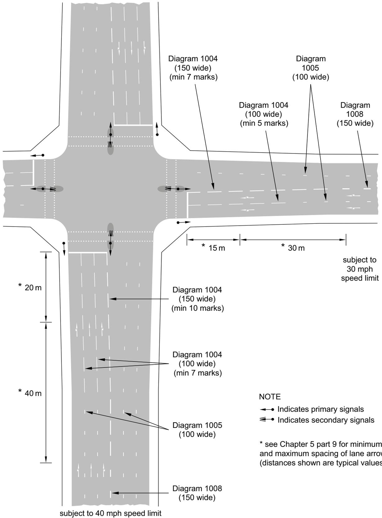
**Figure 4-1** Layout of urban signal junction
