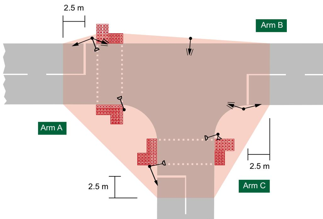
**Figure 2-2** Diagram showing a Junction Intervisibility Zone (with crossings) in relation to the road layout
