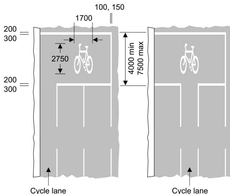
**Figure 12-13** Diagram 1001.2 (S14-2-48): ASL with near side or central approach lane
