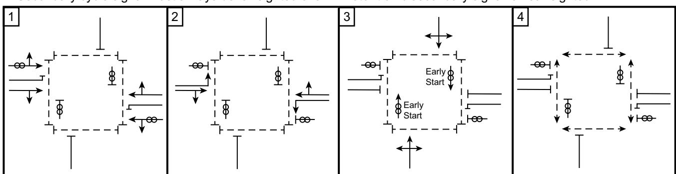
**Figure 12-8** Diagram showing indicative layout and staging for a 'hold the left turn' arrangement at a signal junction
