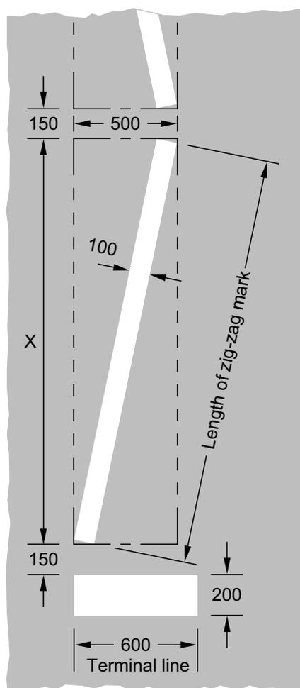
**Figure 15-3** Dimensions of zig-zag line
