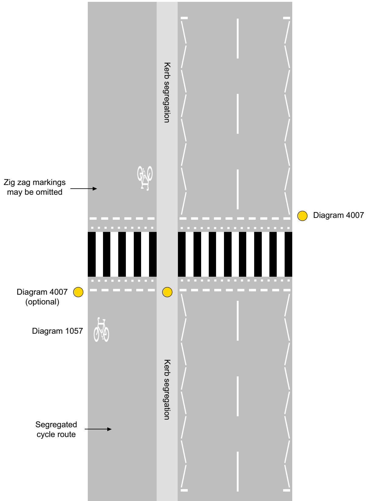
**Figure 15-1** Diagram showing road marking layout for a Zebra crossing across both general traffic lanes and a cycle track
