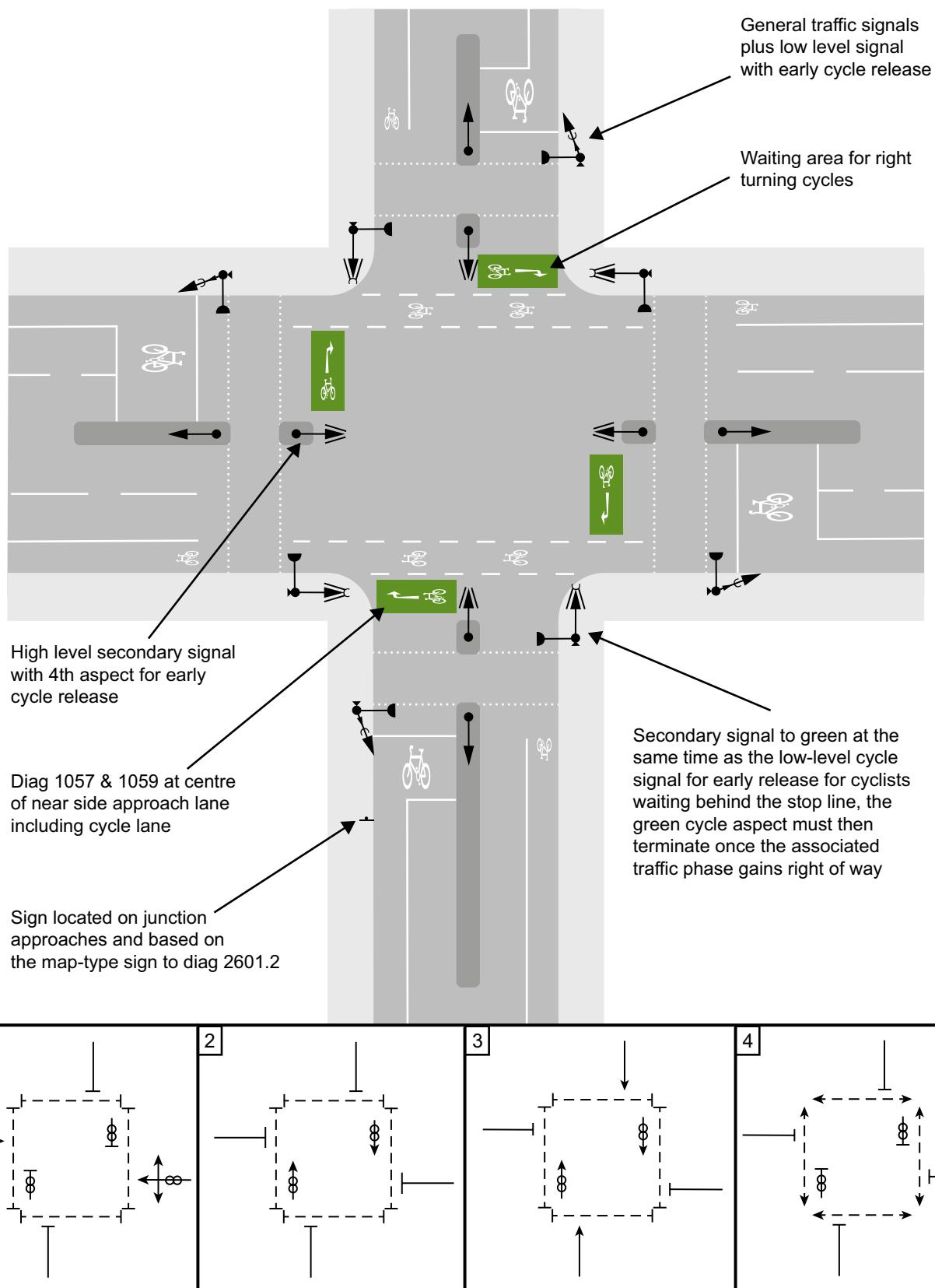
**Figure 12-9** Diagram showing indicative layout and staging for a two-stage right turn arrangement at a signal junction
