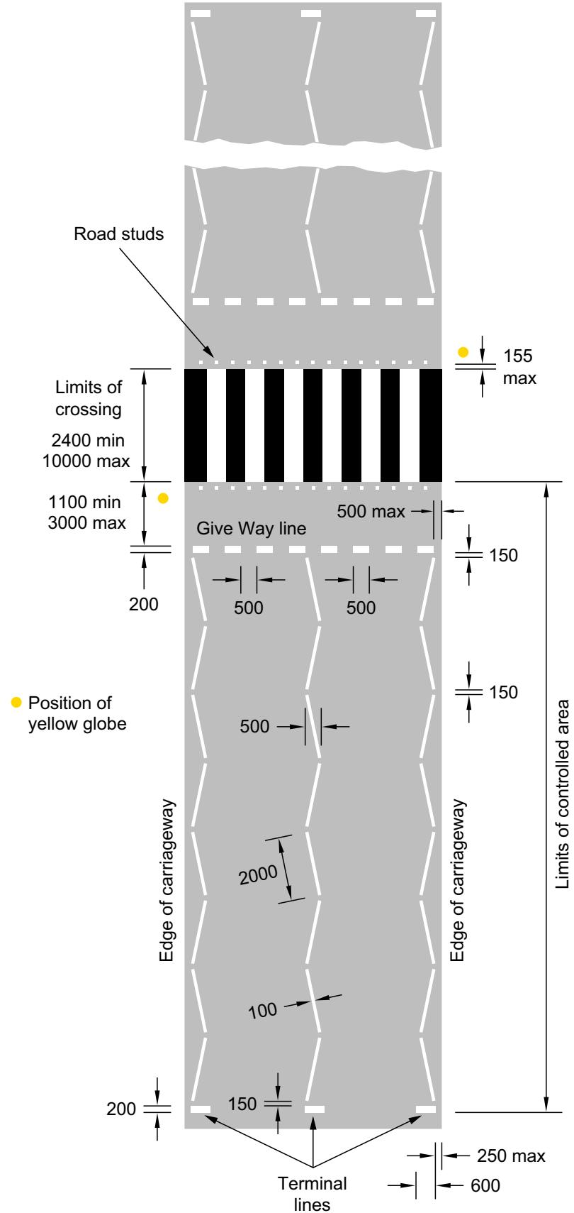
**Figure 16-2** Diagram 1001.4 (S14-2-52): Road markings indicating a Zebra crossing
