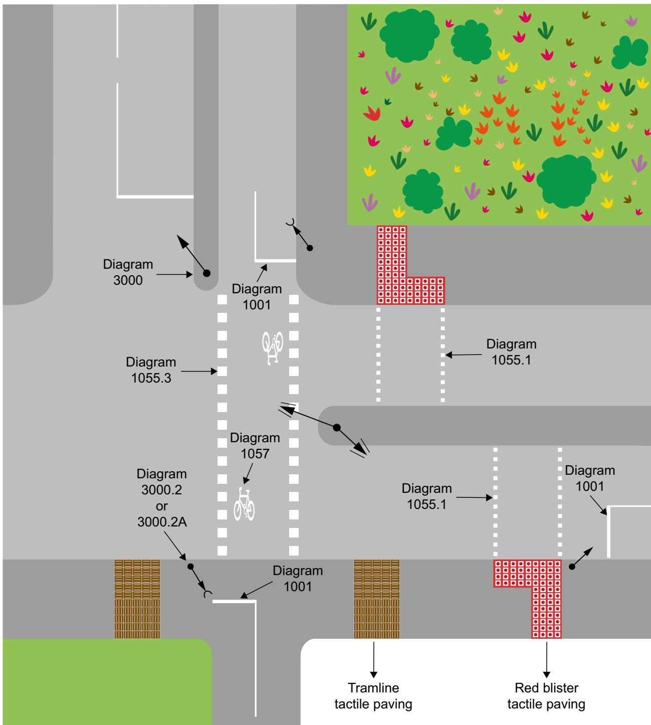
**Figure 12-7** Signalised separate pedestrian and cyclist facility at a junction
