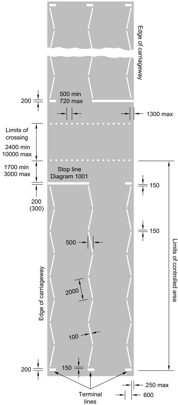
**Figure 15-4** Zig-zag layout for a crossing on a two-way street. The central zig-zag line may be reversed
