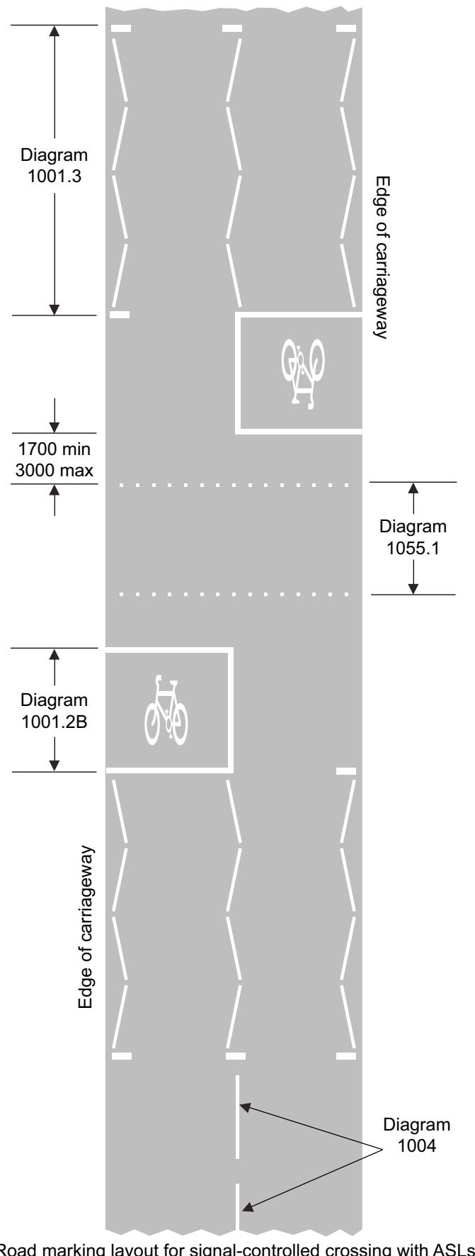
Road marking layout for signal-controlled crossing with ASLs
