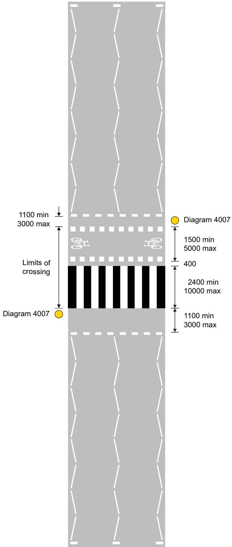
**Figure 17-1** Diagram 1001.5 (S14-2-53): Road markings indicating a Parallel crossing
