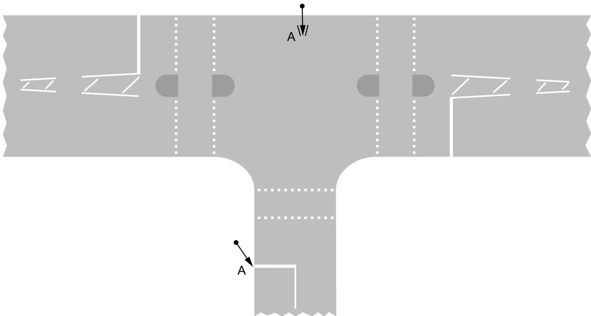
**Figure 3-1** Layout diagram showing the positions of a primary signal head, plus a secondary signal head placed on the far side of the junction
