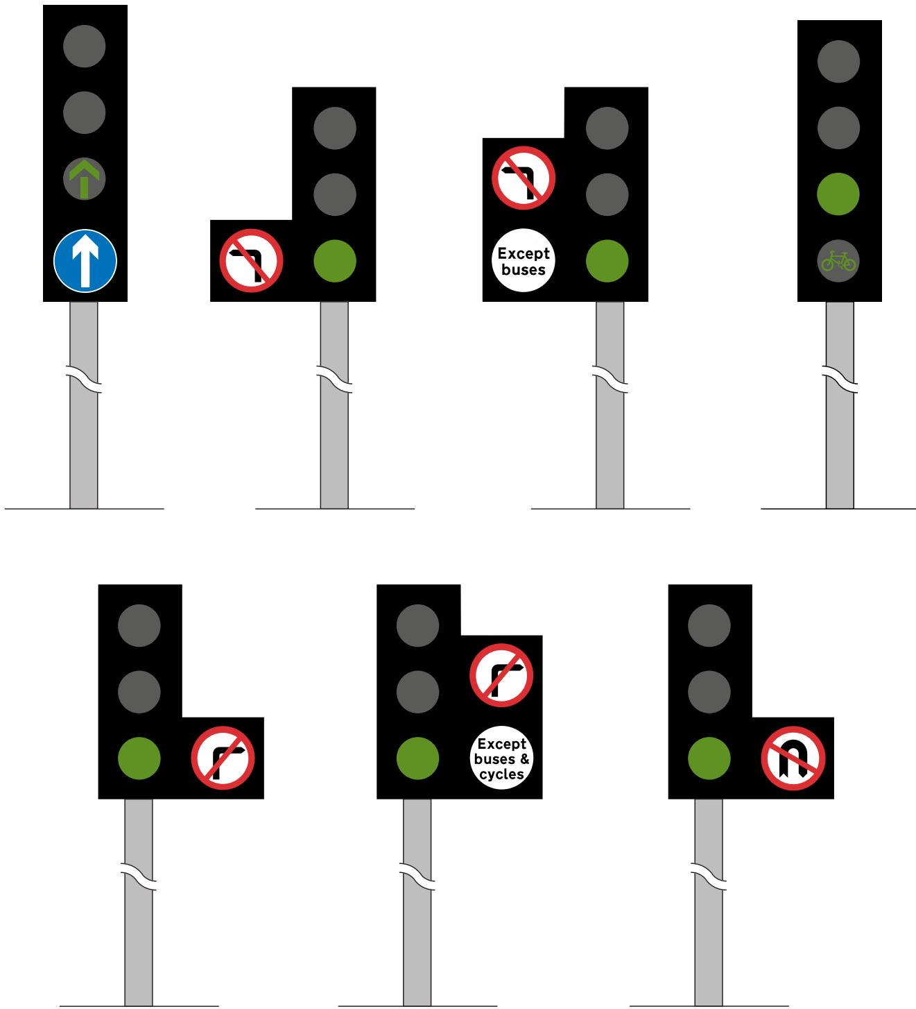
**Figure 5-1** Alternative signal head layouts showing common regulatory box sign arrangements and exception plates
