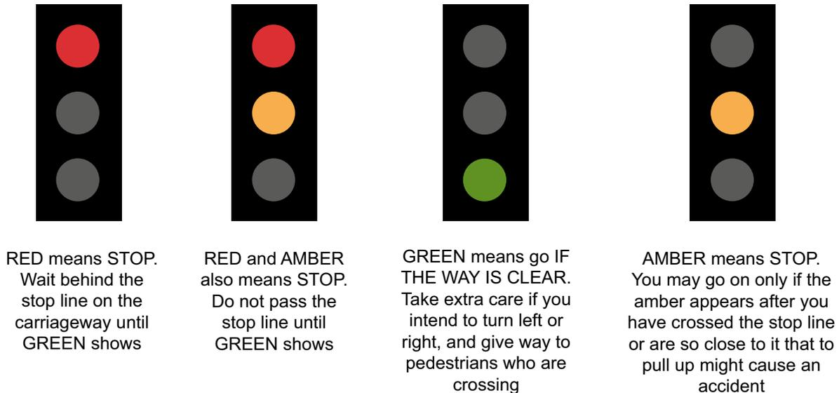
**Figure 6-1** Vehicular traffic signal sequence
