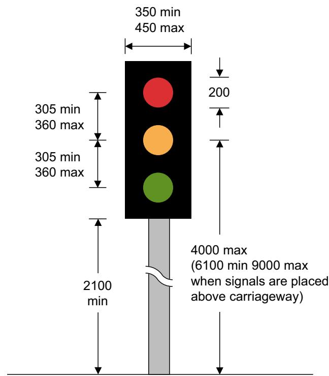
**Figure 3-5** Diagram 3000 (S14-2-1) Permanent traffic signal head
