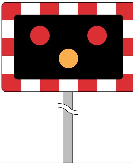
**Figure 24-1** Diagram 3014 (S14-2-5) Wig-wag signal
