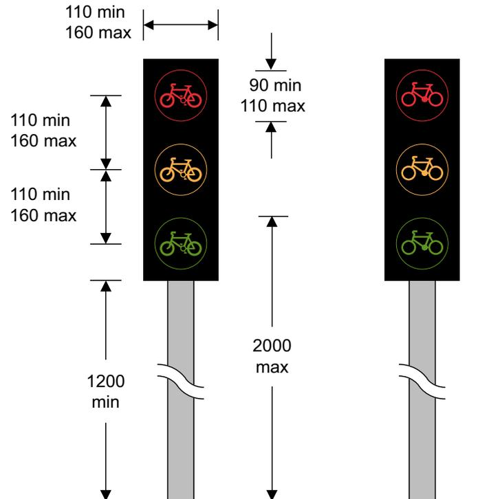
**Figure 12-3** Diagram 3000.2A (S14-2-4): alternative types
