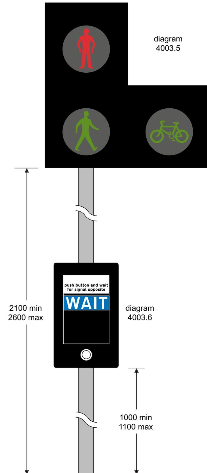
**Figure 12-6** Diagram 4003.5 (S14-2-19) and Diagram 4003.6 (S14-2-20)
