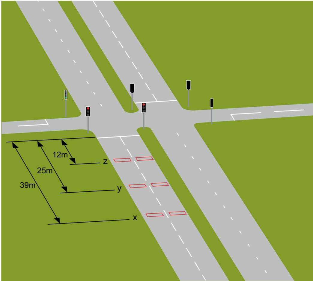
**Figure 10-1** Layout of X, Y and Z detector loops for System D
