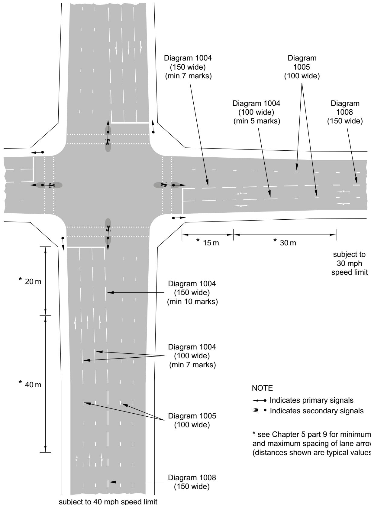
**Figure 4-1 Layout of urban signal junction**
