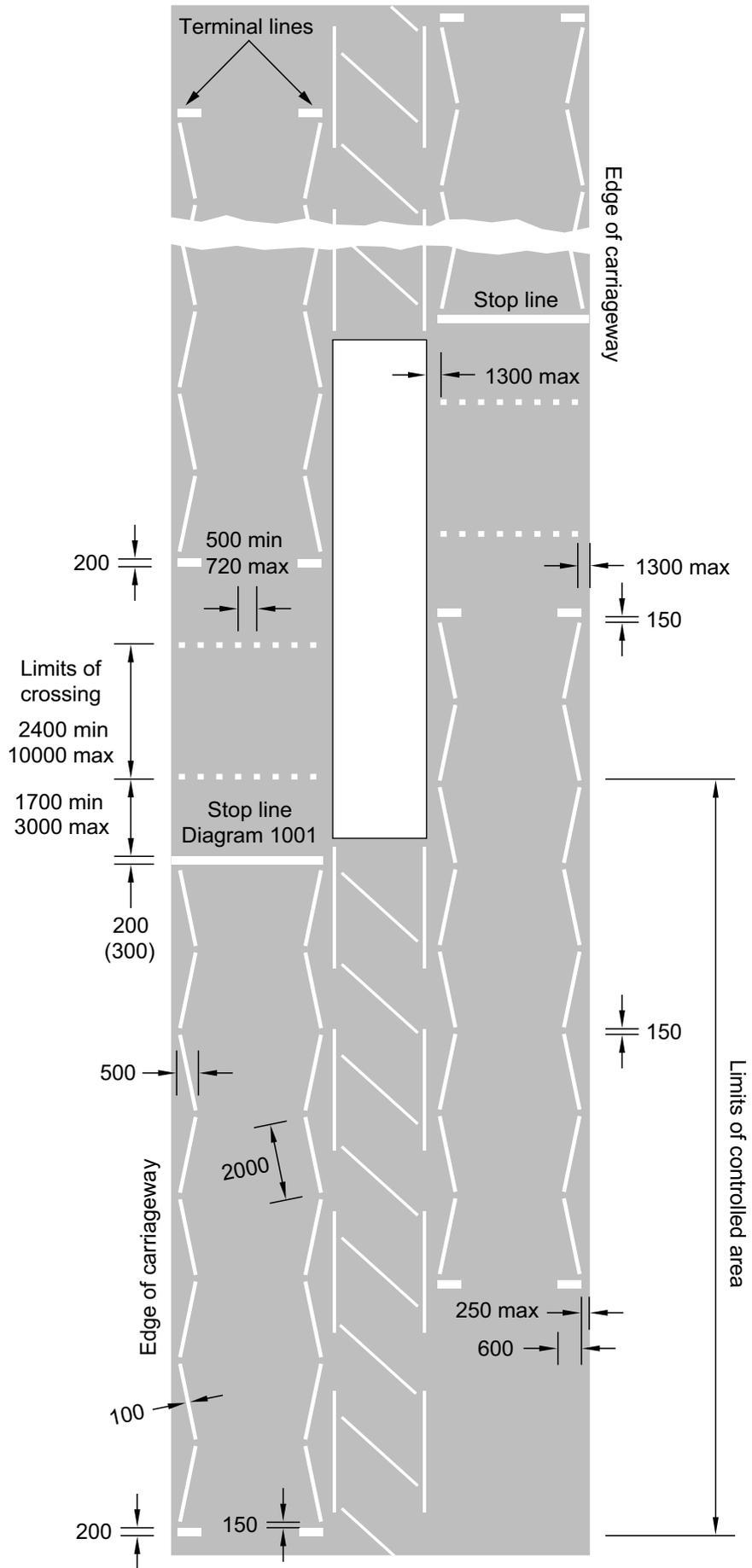
**Figure 15-6** Zig-zag layout for a staggered crossing with a central refuge, incorporating markings to diagram 1040
