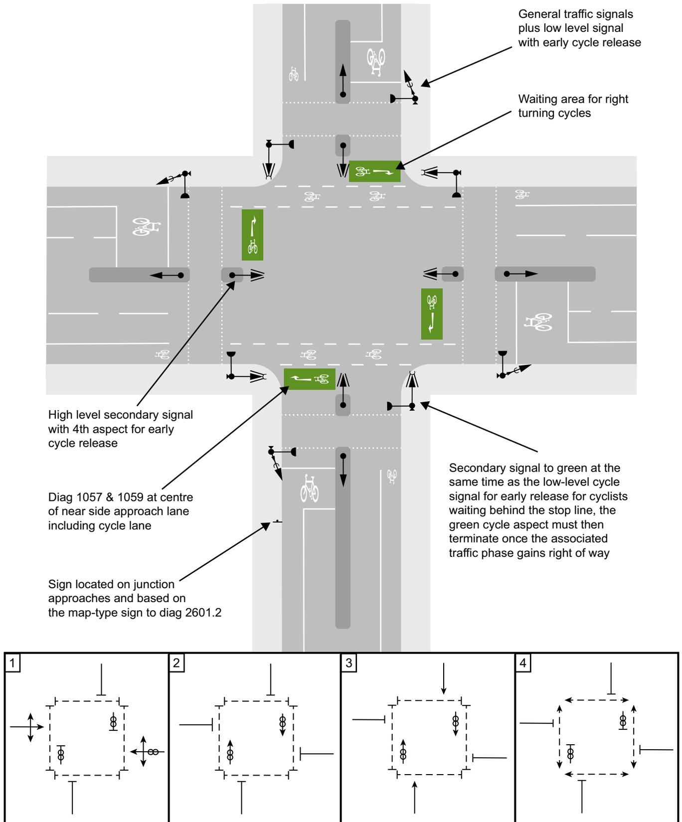
**Figure 12-9** Diagram showing indicative layout and staging for a two-stage right turn arrangement at a signal junction
