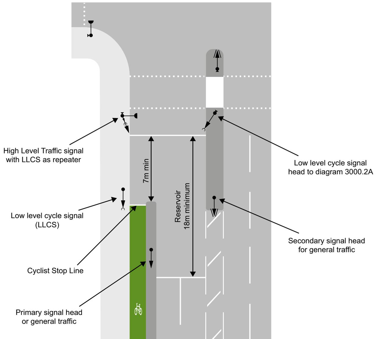
**Figure 12-10** Diagram showing indicative layout of cycle gate road markings and position of signal heads
