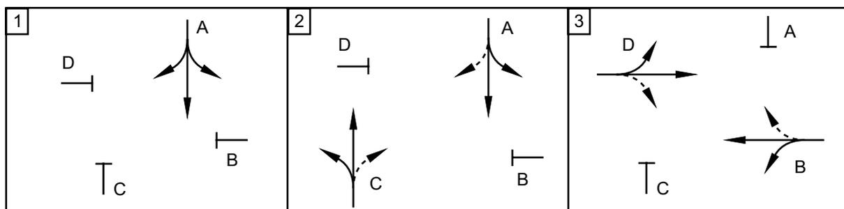
Figure 8-3 Staging diagram showing a late start sequence
