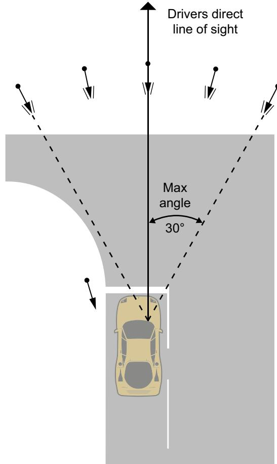
**Figure 3-4** Layout diagram showing the recommended angle of position of secondary signal heads relative to a car positioned at the stop line
