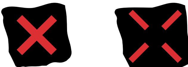
**Figure 26-2** Diagrams 5003 and 5003.1 (S14-2-33) Lane closed to vehicular traffic (Alternative types)
