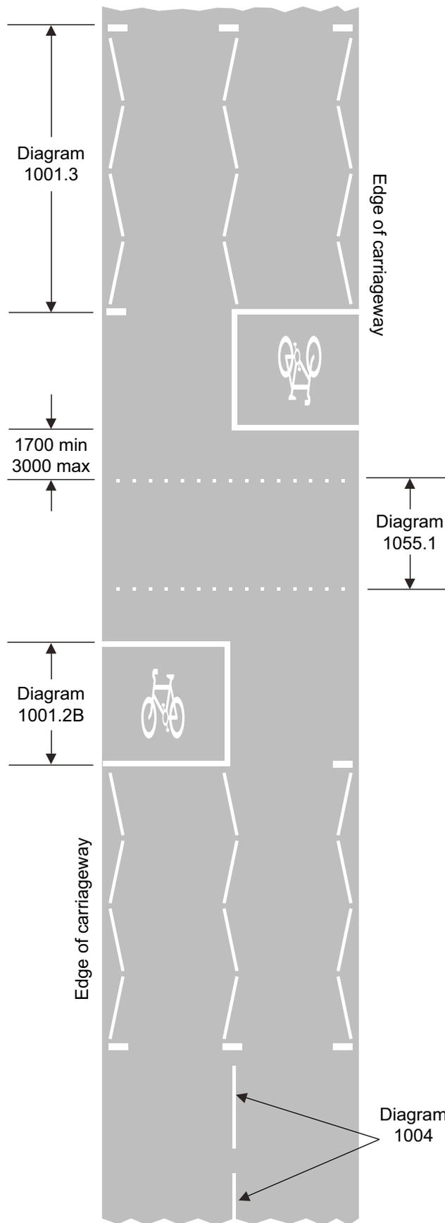
Road marking layout for signal-controlled crossing with ASLs
