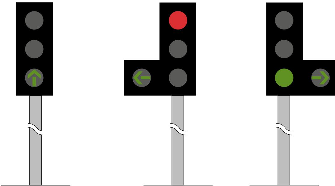
**Figure 3-6** Diagrams showing alternative signal head arrangements incorporating, from left to right, a substitute green arrow, a left turn filter arrow, and a right turn indicative green arrow.
