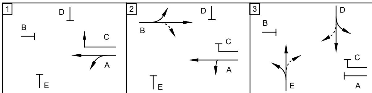
**Figure 8-2** Staging diagram showing a separately signalled right turn sequence
