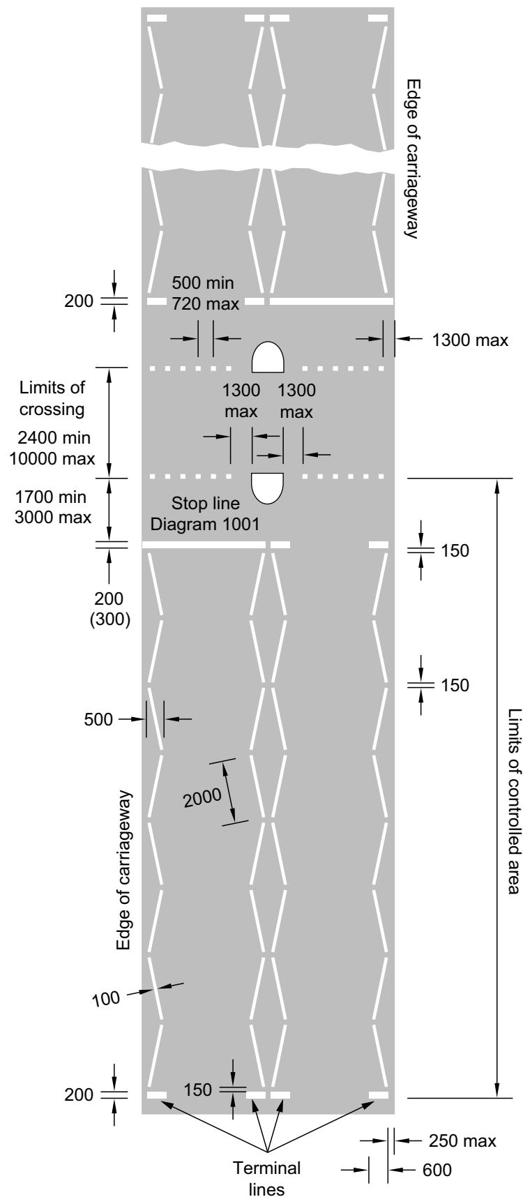
**Figure 15-5** Zig-zag layout for a crossing on a two-way street with a central refuge island
