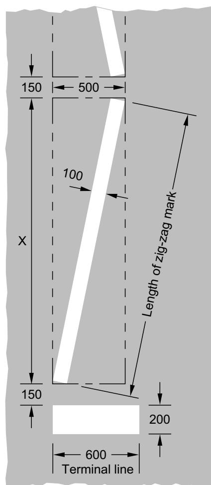
**Figure 15-3** Dimensions of zig-zag line
