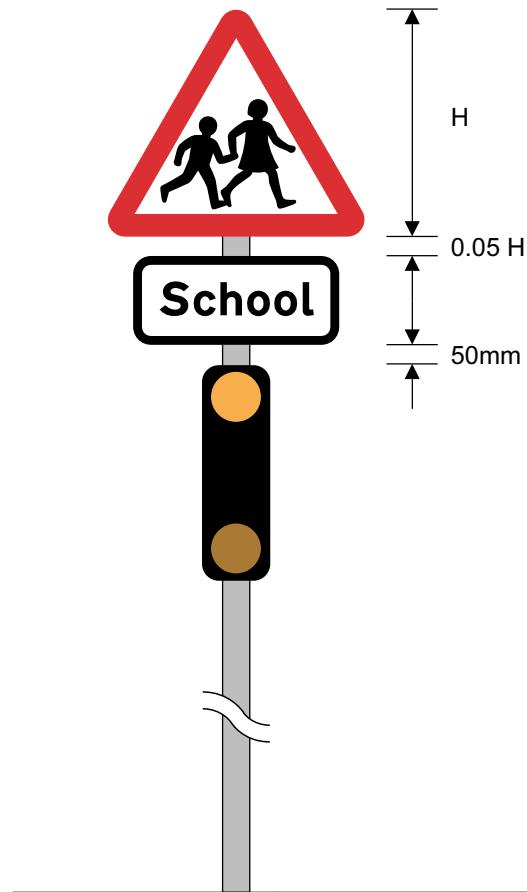
**Figure 25-1** Diagram 545 (S2-2-25) and associated plate, shown in combination with diagram 4004 (S14-2-23)
