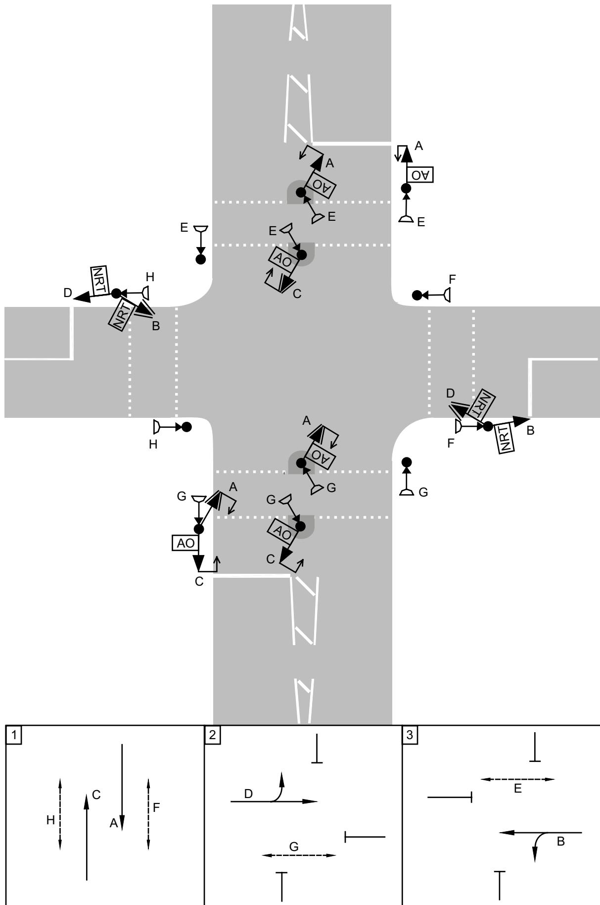
**Figure 11-5** Walk with traffic pedestrian facility
