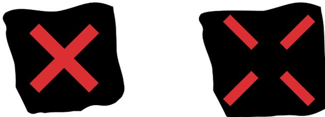
**Figure 26-2** Diagrams 5003 and 5003.1 (S14-2-33) Lane closed to vehicular traffic (Alternative types)
