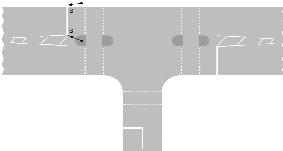
**Figure 3-2** Layout diagram showing the positions of a primary signal head, plus a double or duplicate primary signal head
