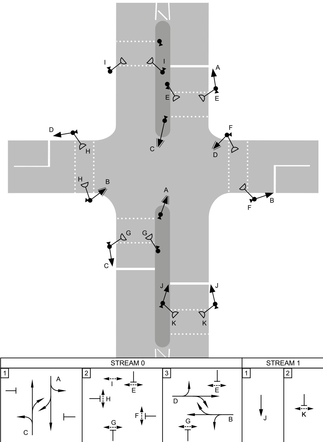
**Figure 11-6** Diagram showing indicative layout of a staggered pedestrian facility
