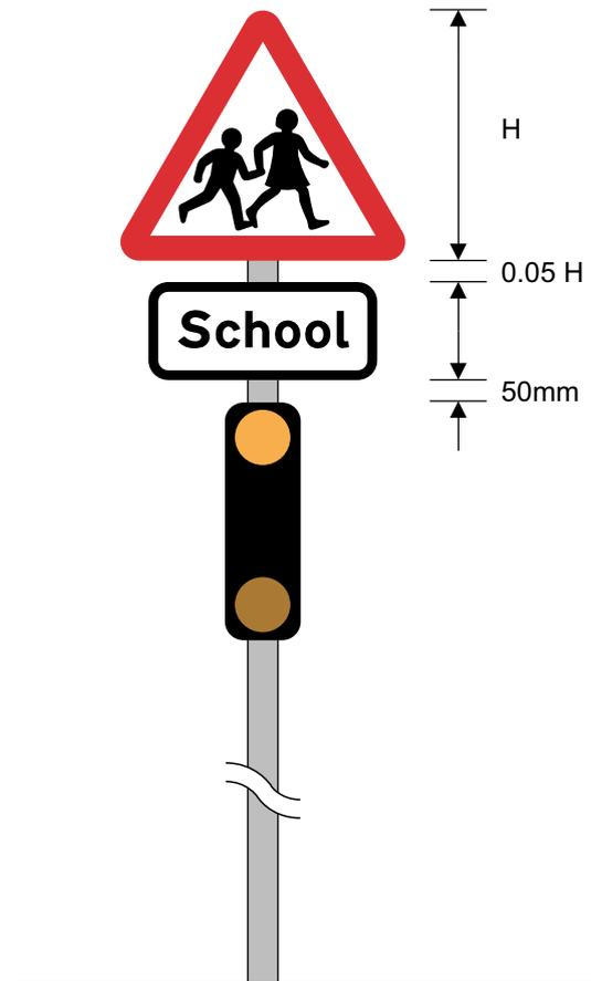
**Figure 25-1** Diagram 545 (S2-2-25) and associated plate, shown in combination with diagram 4004 (S14-2-23)
