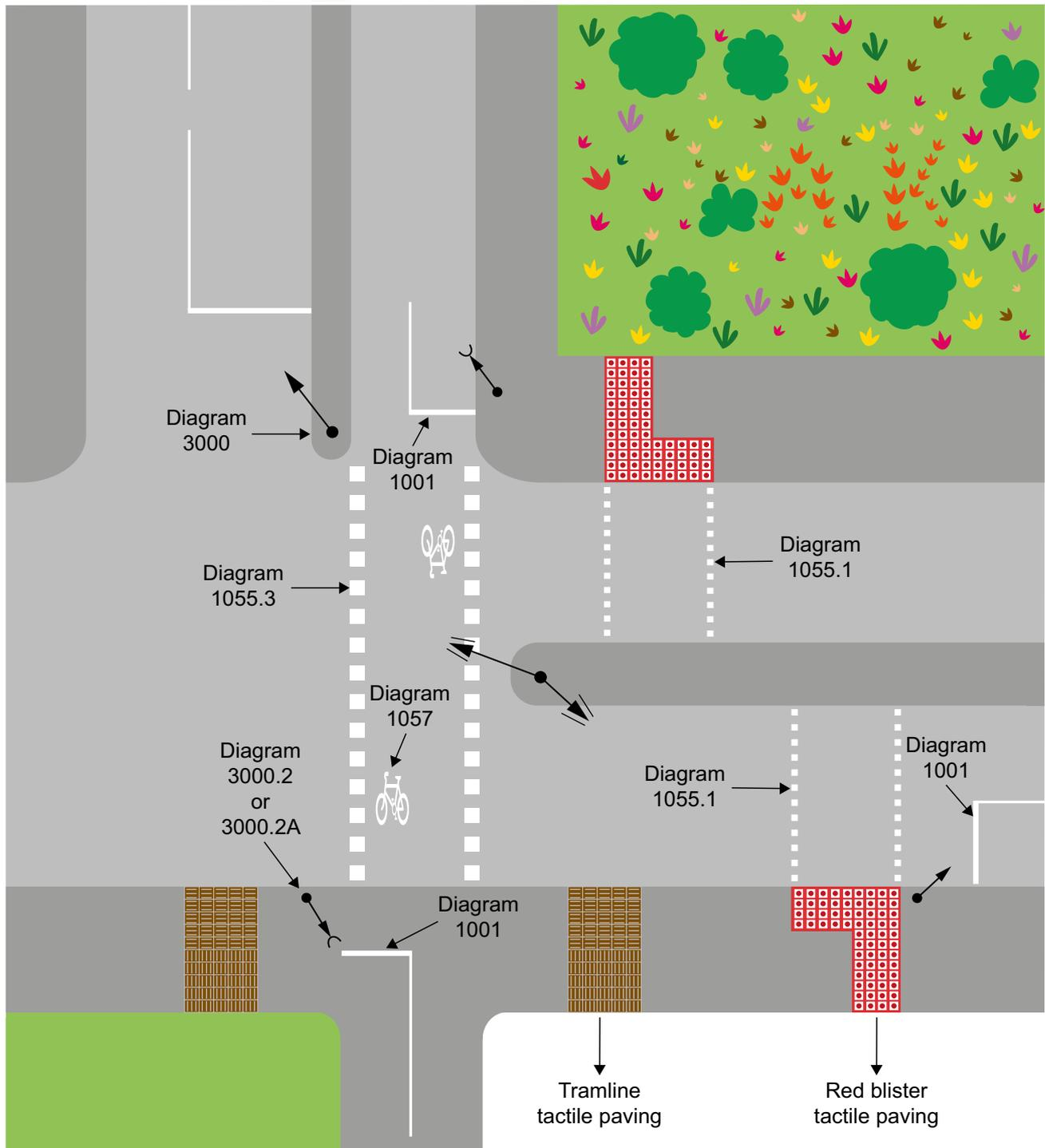
**Figure 12-7** Signalled separate pedestrian and cyclist facility at a junction
