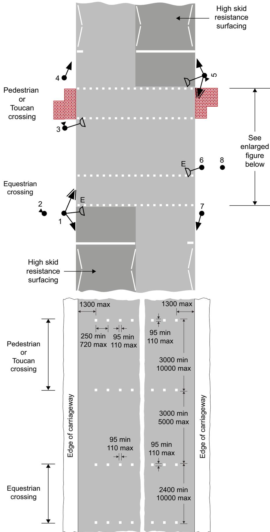
**Figure 22-1** Layout of a parallel equestrian and pedestrian or Toucan facility
