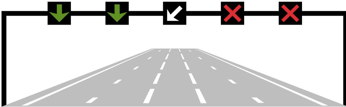
**Figure 26-3** Example of lane control signals mounted above the carriageway for a tidal-flow system
