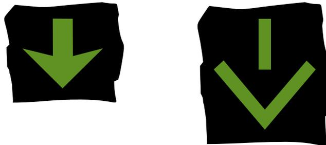
**Figure 26-1** Diagrams 5001.1 and 5001.2 (S14-2-32) Lane open to vehicular traffic (Alternative types)
