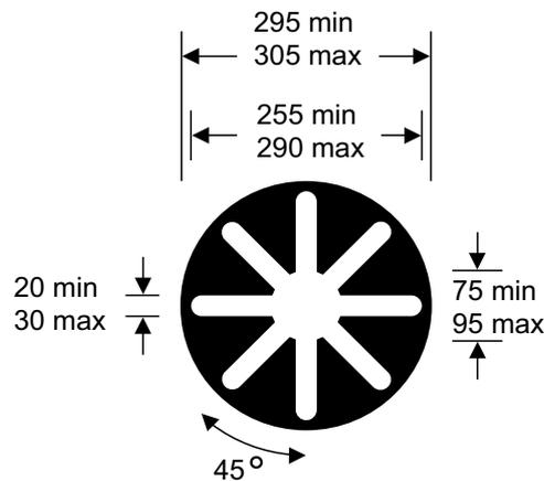
**Figure 23-1** Diagram 3013 (S14-3-2) Light signal for control of tramcars
