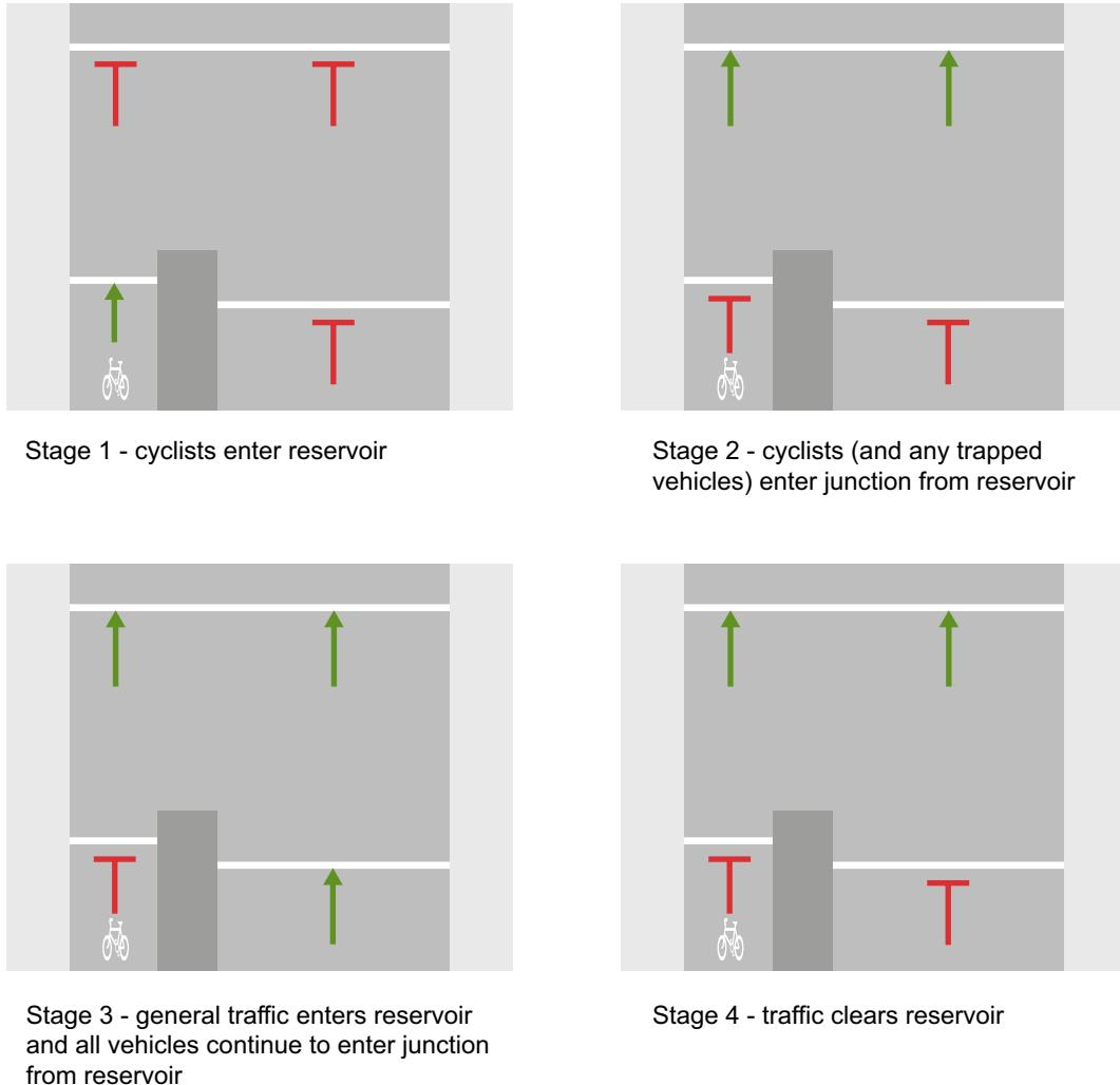
**Figure 12-11** Diagram showing operational sequence for a cycle gate facility
