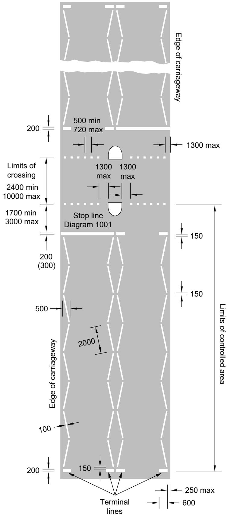
**Figure 15-5** Zig-zag layout for a crossing on a two-way street with a central refuge island
