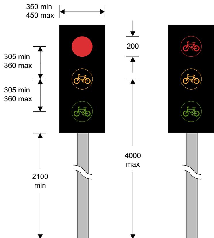
**Figure 12-2** Diagram 3000.2 (S14-2-3), alternative types
