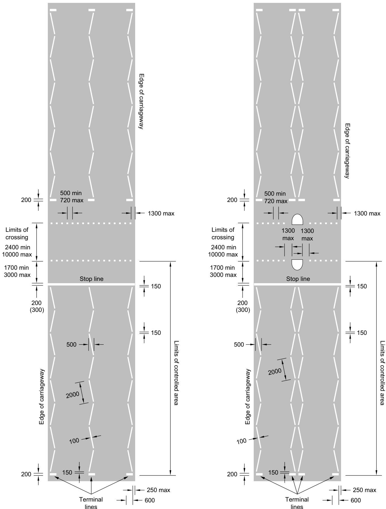
**Figure 15-7** Zig-zag layout for signal-controlled crossings on one-way streets, with and without a central refuge island
