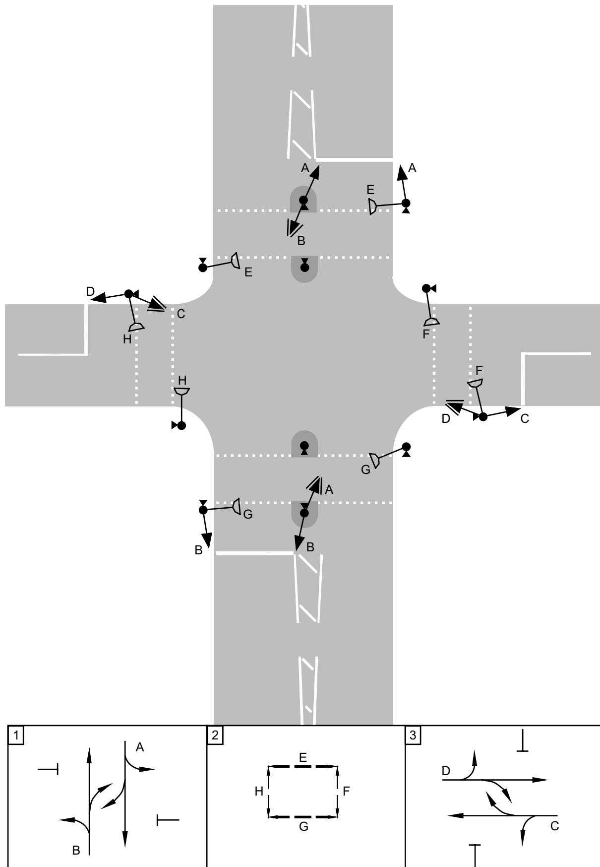
**Figure 6-2** Layout diagram showing phases and stages for a crossroads junction with a full pedestrian stage
