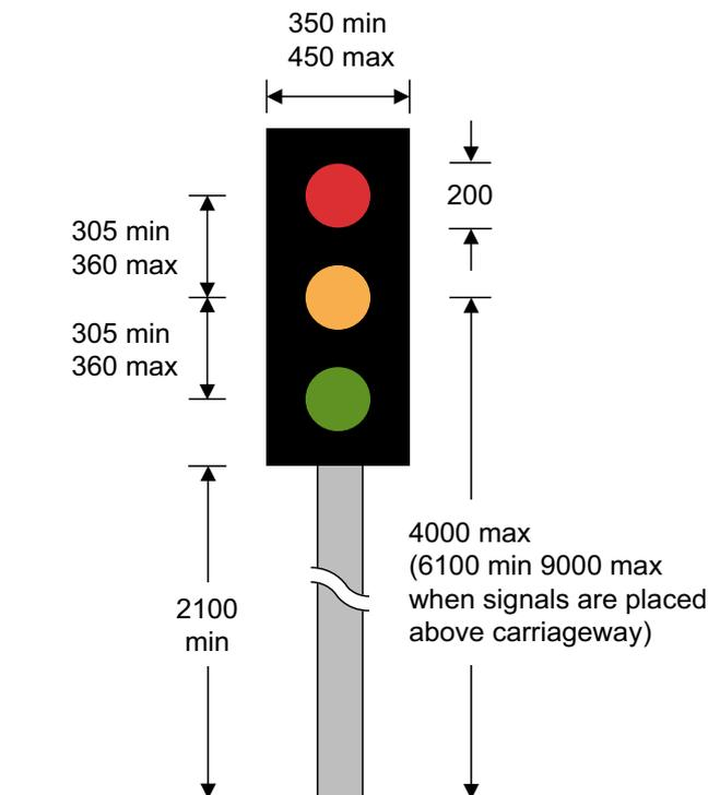
**Figure 3-5** Diagram 3000 (S14-2-1) Permanent traffic signal head
