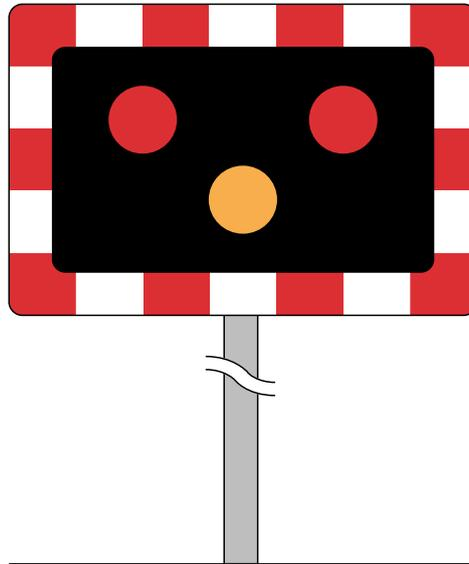
**Figure 24-1** Diagram 3014 (S14-2-5) Wig-wag signal
