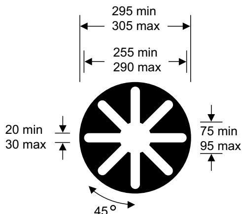
**Figure 23-1** Diagram 3013 (S14-3-2) Light signal for control of trams
