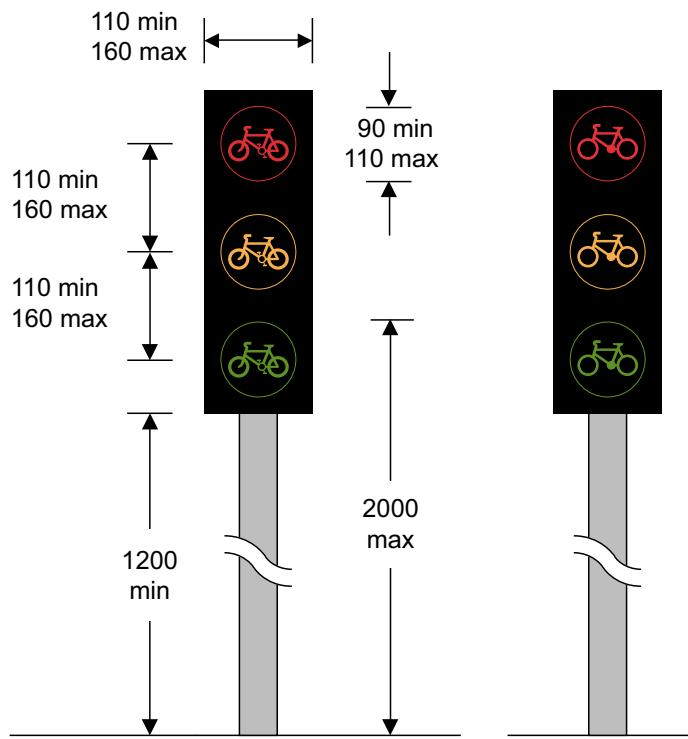
**Figure 12-3** Diagram 3000.2A (S14-2-4): alternative types
