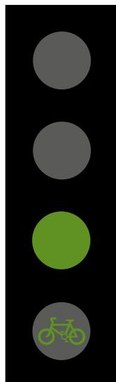
**Figure 12-12** Diagram 3001.4: green cycle aspect as an additional aspect to vehicle signals to diagram 3000
