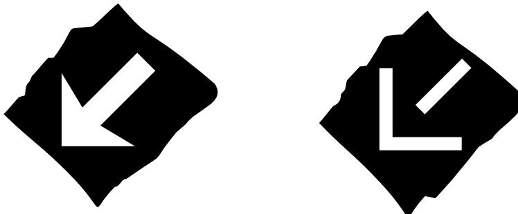
**Figure 26-4** Diagrams 5005 and 5005.1 (S14-2-34) Lane closed ahead and vehicular traffic should move to the next lane on the left (Alternative types)
