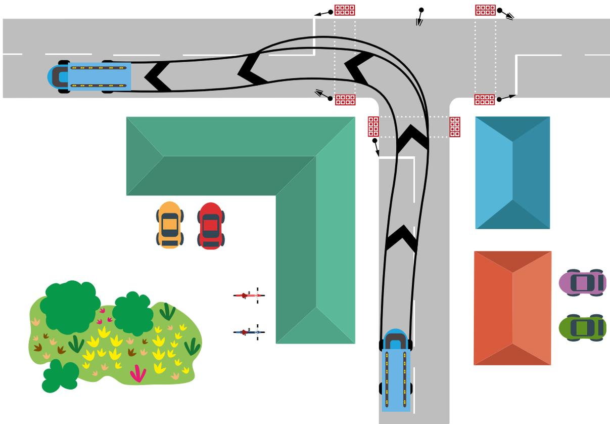
**Figure 2-3** Despite the small corner radius, with sufficient carriageway width a long vehicle can still negotiate a junction
