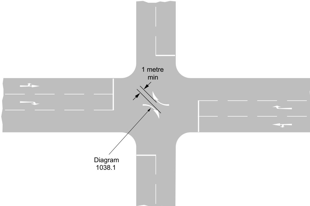
**Figure 4-2** Layout of guidance arrows at a signal-controlled junction
