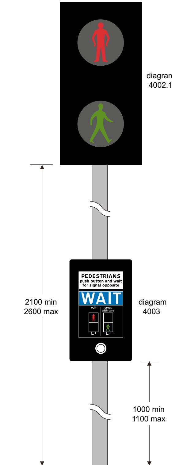
Mounting arrangement for pedestrian signal head to diag 4002 and push button to diag 4003. Similar arrangements should be used for farside toucan crossings. Diag 4003.8 may be used instead of diag 4003; the same height is recommended.
