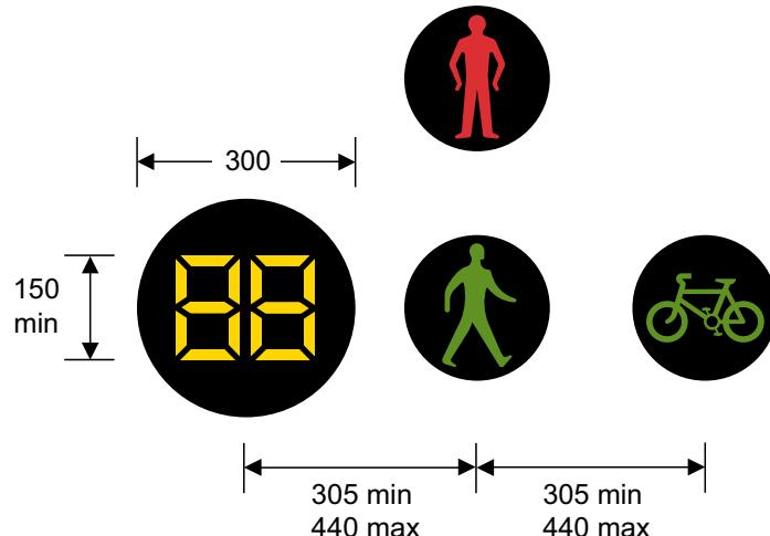
**Figure 11-4** Diagram 4002.1A (S14-2-10) Pedestrian countdown unit, shown in combination with the diagram 4003.5 (S14-2-19)
