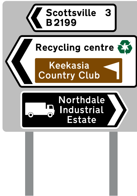
Figure 7-1 Effective use of backing boards
